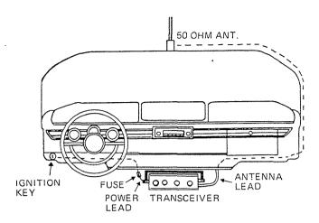
Connect the antenna plug to the antenna jack with an SWR-Meter inserted into the antenna cable.
